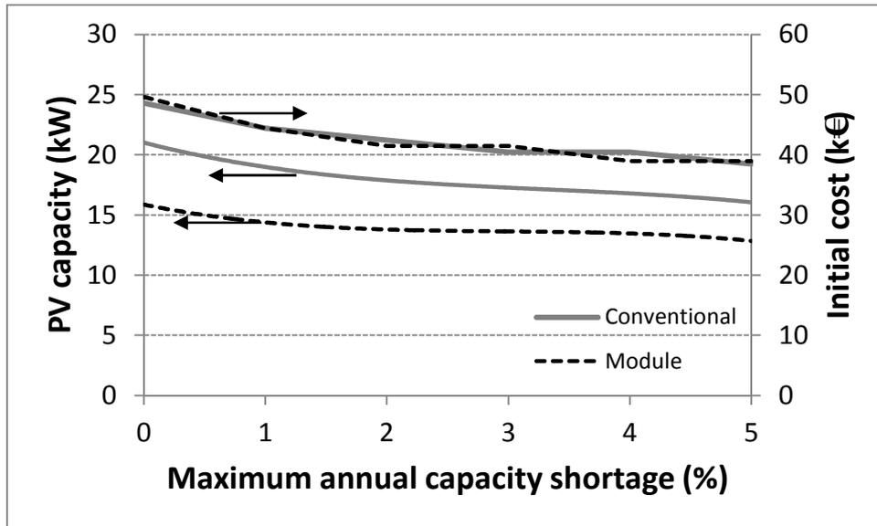
**Figure 8.** Required capacity of PV array for various acceptable values of annual capacity shortage, and respective initial cost of the system for 20€/m<sup>2</sup> assumed reflectors cost.
