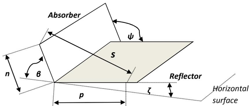
**Figure 2.** Design parameters of the examined PV/reflector arrangement
