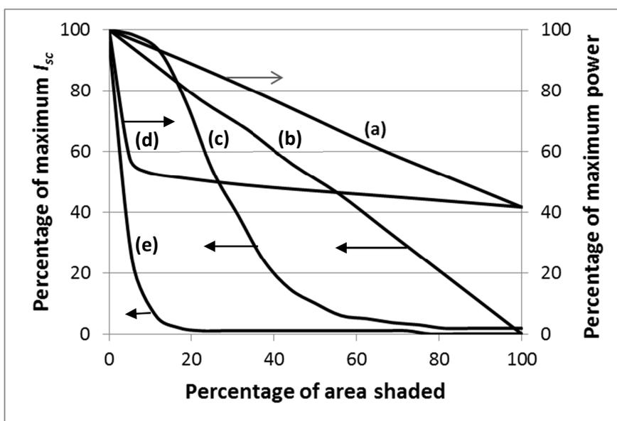
**Figure 4.** Effect of shading on mono-crystalline and amorphous silica PV panels. (a, b): Shading of *a-Si* vertically to the cells, (c, d): Shading of *a-Si* in parallel to the cells, (e): Shading of *m-Si* panel. Curves (a) and (d) refer to 60% shading, all other to complete shading
