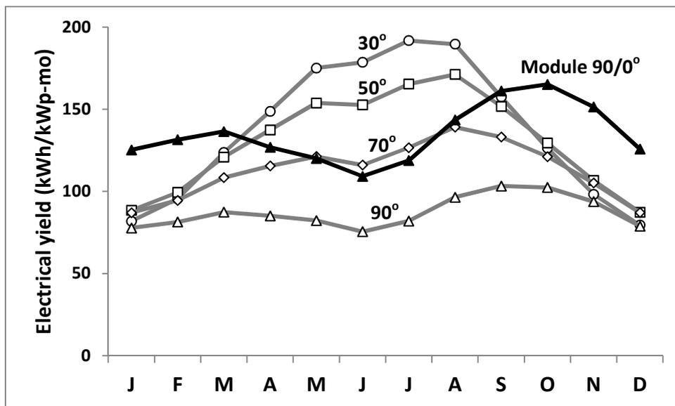
**Figure 7.** Expected electrical yield of PVs for various tilt angles (at 30°, 50°, 70° and 90°), as compared to the yield from a PV/reflector module (at  $\beta=90^\circ$ ,  $\zeta=0^\circ$ ,  $p/n=2.0$ ).
