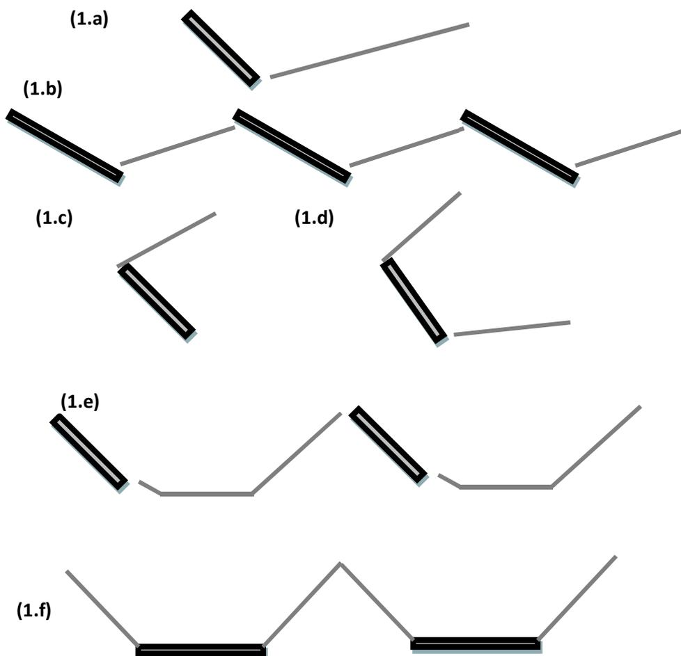
**Figure 1.** Various tested arrangements of flat booster reflectors with PVs. (a) Single unit, (b) Same as previous, but in arrays, (c) Reflector on top of the PV to protect it from snow, (d) With two reflectors at a single unit (trough arrangement), (e) With two reflectors in arrays (floating unit), the one mirror at horizontal position, (f) With two reflectors in arrays, (floating unit), the PV at horizontal position for cooling.
